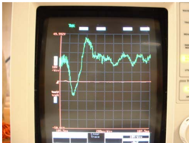
Figure 9: PEP-II e+ Beam Measured by the Single-Shot Scope
