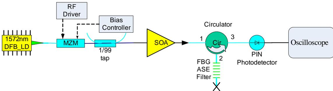
**Figure 1.** Measurement setup.
