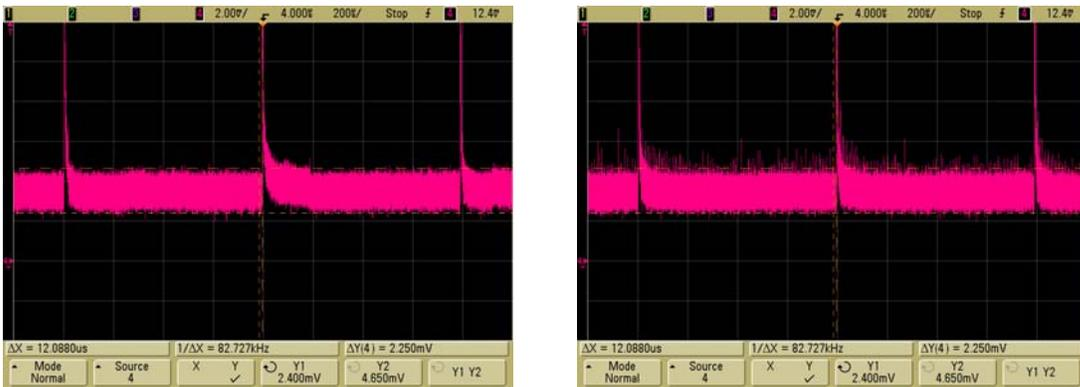
**Figure 4.** Screen shot of the leakage power under 1.25kHz pulsed operation ( $PW=0.96\mu\text{s}$ ,  $\text{Period}=887\mu\text{s}$ ) when biased at a null point with laser on and SOA on ( $I = 500\text{mA}$ ): (*left*) using the bias card; (*right*) biased manually. For both cases, the leakage is the same as the CW operation.
