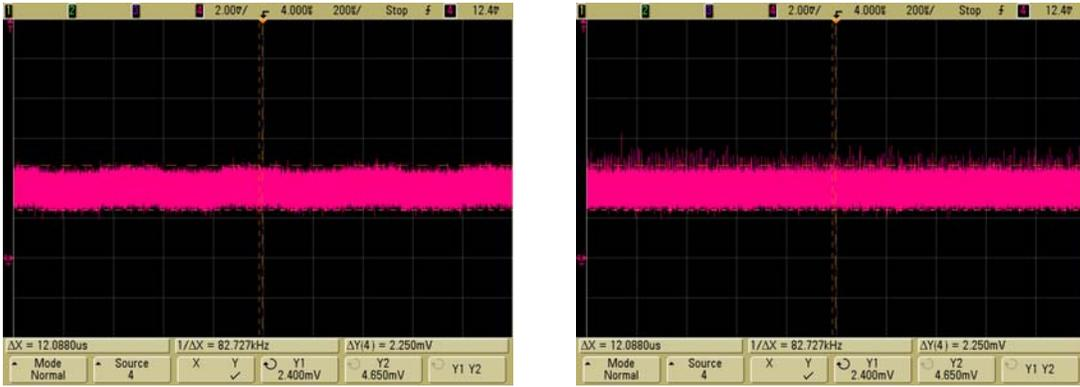
**Figure 3.** Screen shot of the leakage power when biased at a null point under CW operation with laser on and SOA on ( $I = 500\text{mA}$ ): (*left*) using the bias card; (*right*) biased manually.
