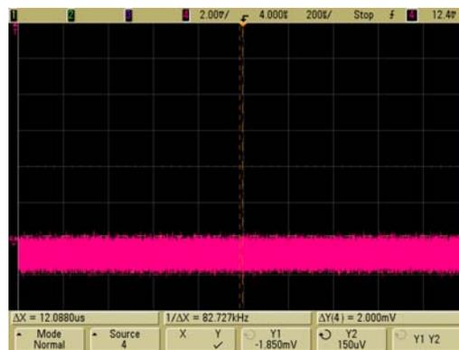
**Figure 2.** Detector noise floor without optical signal ( $V_{min} = -1.85mV$ ,  $V_{max} = 0.15mV$ ,  $V_{peak\_peak} = 2.0mV$ ,  $V_{average} = -0.85mV$ ).
