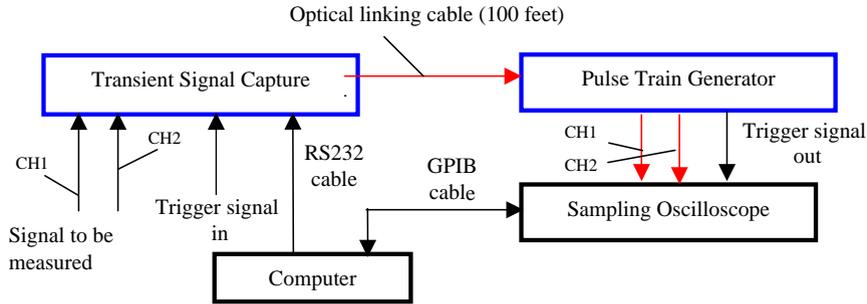
Fig. 3. Fiber Loop Single-Shot Scope configuration. CH, channel.
