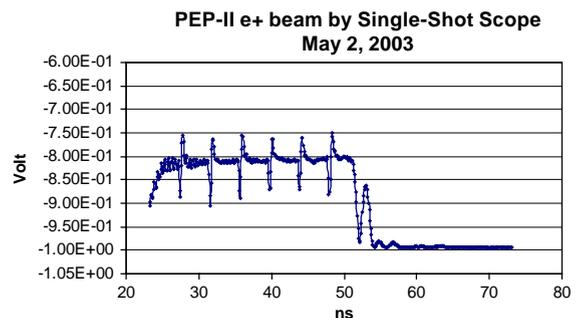
Fig. 8. Measurement of  $e^+$  bunches captured by the Fiber Loop Single-Shot Scope.
