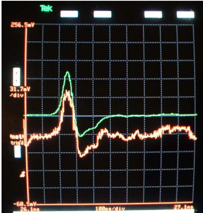
Fig. 11. The measured signal (bottom) and the original signal (top).
