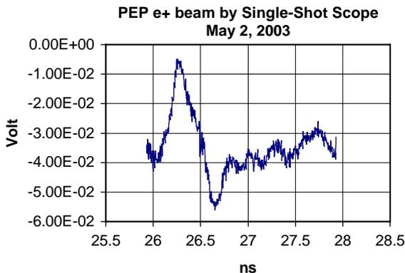
Fig. 6. PEP-II  $e^+$  beam bunch longitudinal distribution measured with the Fiber Loop Single-Shot Scope.
