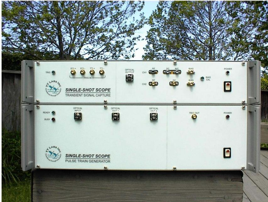
Fig. 1. YY Labs' Fiber Loop Single-Shot Scope.
