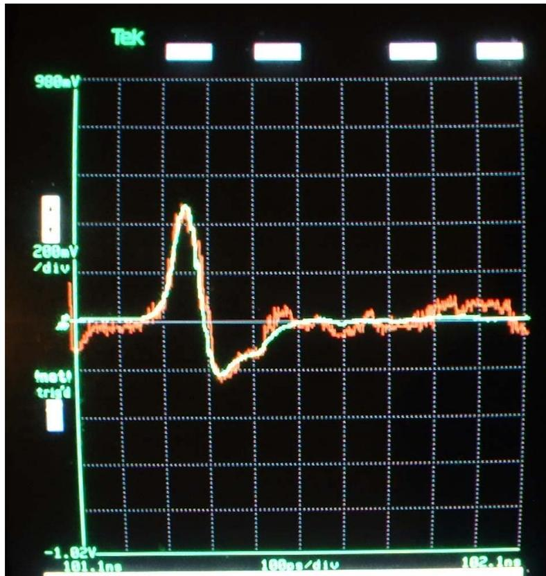
Fig. 10. The overlapped original signal (front) and measured signal (back).
