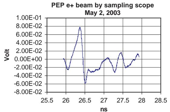
Fig. 7. PEP-II  $e^+$  beam bunch average longitudinal distribution measured directly with the TEK 11801 sampling scope.
