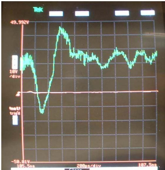
Fig. 9. PEP-II  $e^+$  beam measured by the Fiber Loop Single-Shot Scope.
