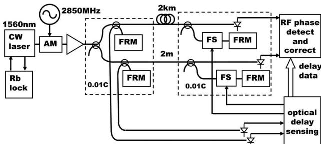
Fig. 2. Dual-channel transmission experiment. The frequency is 2850 MHz.
